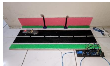
Gambar 4.3 Desain Alat Prototype Sensor LDR
